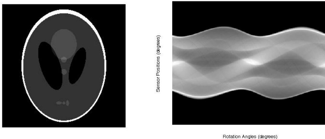
Figure 3: Shepp-Logan phantom (left) and its sinogram (right).
