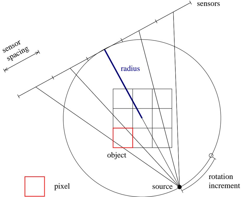
Figure 1: Setup and construction of projection matrix
