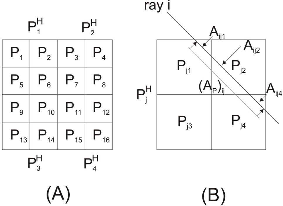
Figure 2: Relation between fine and coarse grid matrix entries.
