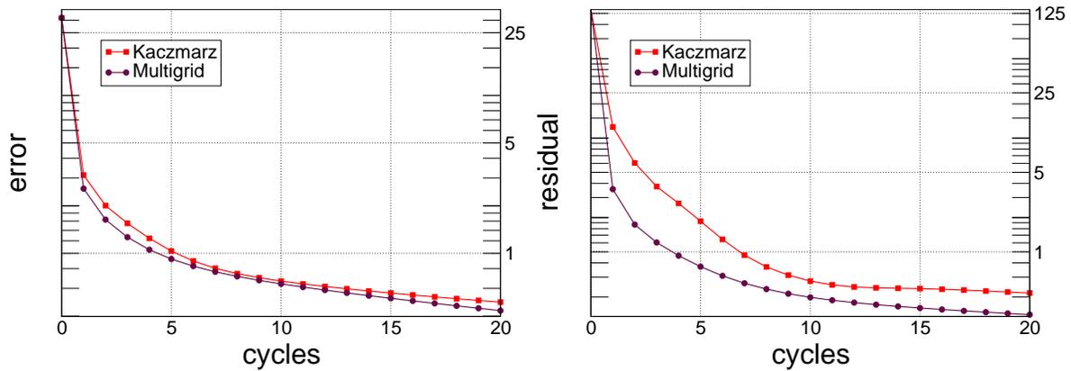
Figure 5:  $L_2$ -norms of errors and residuals for  $V(2,0)$ -cycles using only 1 level (Kaczmarz) and using 2 levels with a direct solver (pseudo inverse) on the coarse grid.
