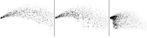
Figure 7: Effect of the drag model for different size scales. The simulations were parametrized to represent scales of 10cm, 1m and 10m, from left to right. The smaller particles, are slowed down, and cause mist below the outflow.
